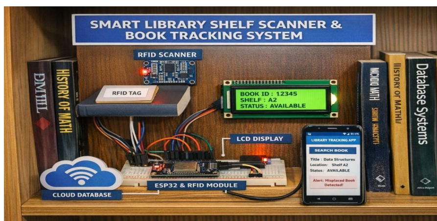
Fig 1. Basic structure of Smart library shelf scanner and book tracking system
