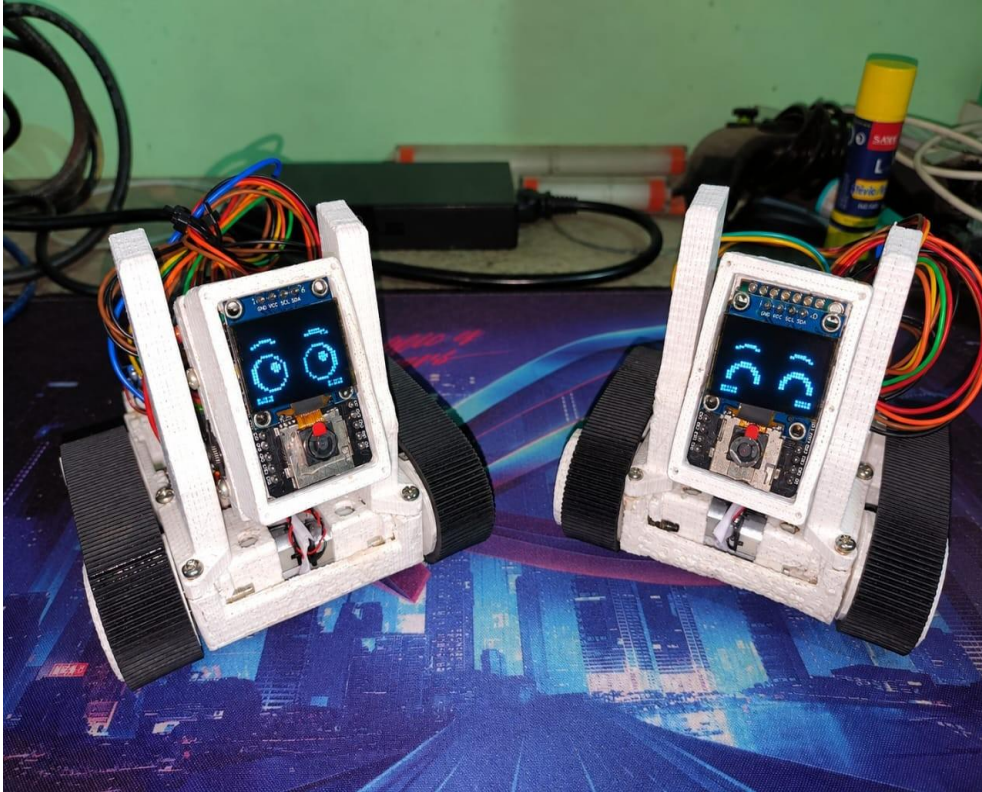
Fig. 10. Assembled prototype of two ESP32-based SKE swarm robots used for experimentation.
