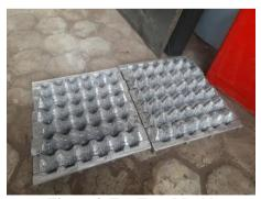
Figure 4: Egg Tray Mould
