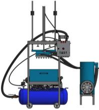
Figure 2: Egg Tray Molding Machine Design (Front View)
