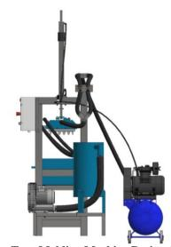
Figure 3: Egg Tray Molding Machine Design (Right View)
