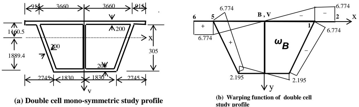
Fig.2 Double cell mono-symmetric study profile and its warping function
