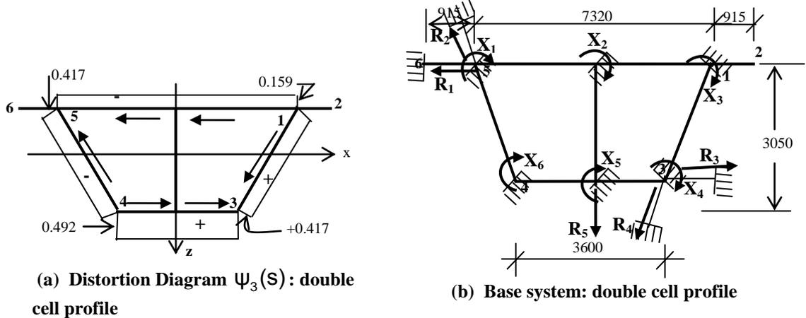
Fig. 4 Distortion diagram and base system for evaluation of distortional bending moment: Double cell study profile
