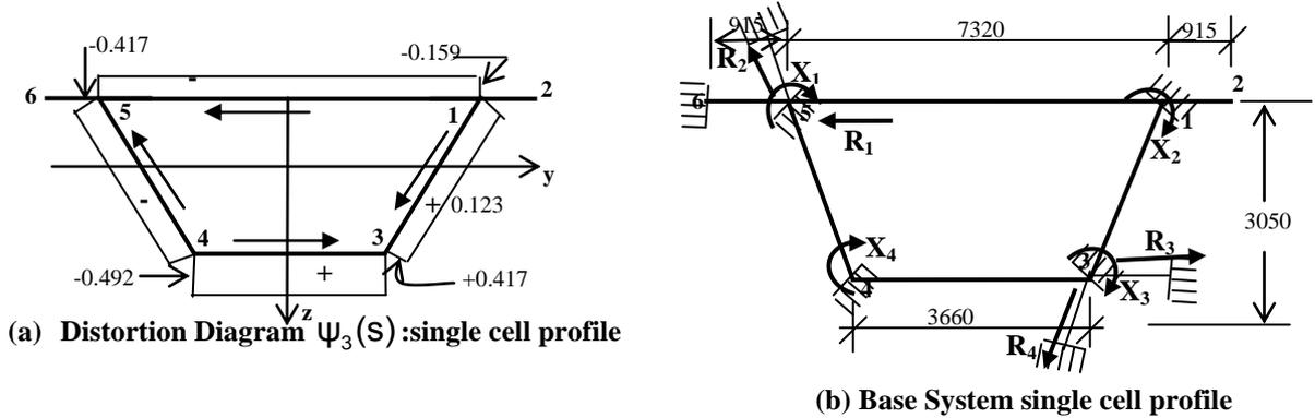
Fig. 3 Distortion diagram and base system for evaluation of distortional bending moment: Single cell study profile
