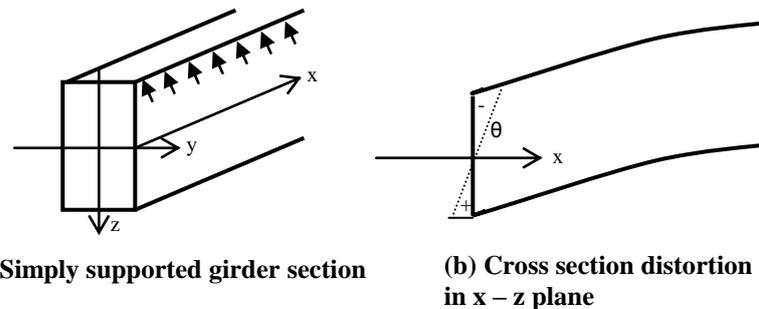
Fig. 7 Simply Supported Girder and Cross Section Distortion
