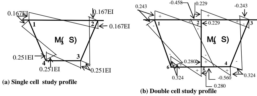
**Fig. 5 Bending moment diagrams due to distortion of mono-symmetric box girder study profiles**
