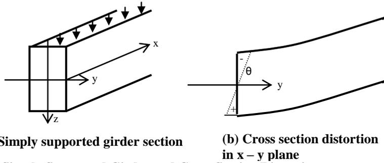
Fig. 6 Simply Supported Girder and Cross Section Distortion
