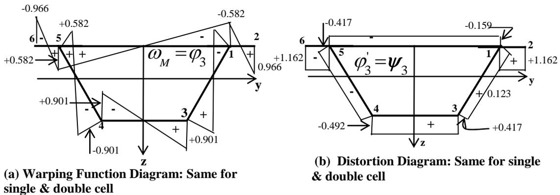
Fig. 8: Warping function and distortion diagrams for single cell and double cell study profiles [5]
