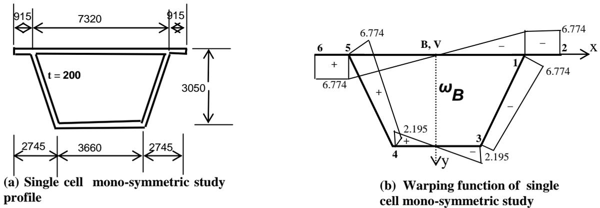
Fig.1 Single cell mono-symmetric study profile and its warping function
