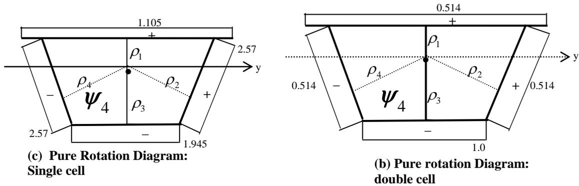
Fig. 9: Rotation diagrams for single cell and double cell study profiles [5]
