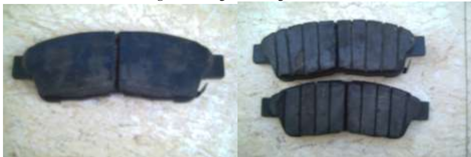
(a) Flat pad used in test
