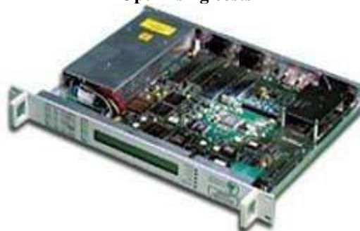
Paradise P300 - cover removed
