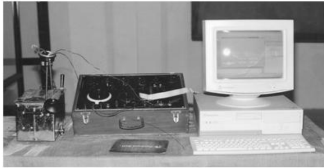
Fig 1: CAX set-up for thermocouple testing
