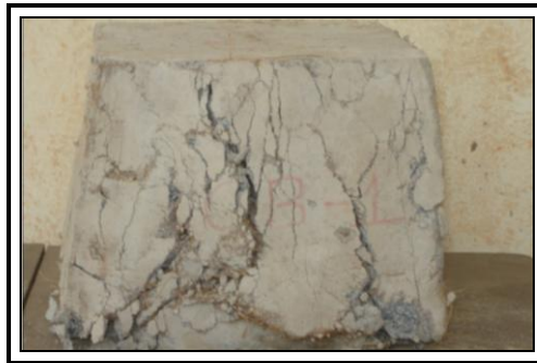
FIG. 5 CUBE AFTER COMPRESSION TEST
