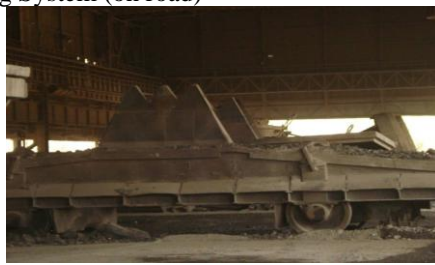
Fig.3 Slag dump car (on track)
