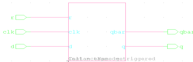
Fig.2: TSPC Edge triggered d flip-flop – symbol
