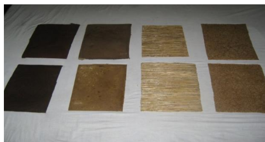
Fig. 2: Bio-Composite Sheet with Different Types of Fibers
