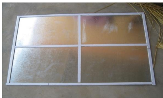
Fig. 1: Layout and Setup of Mould
