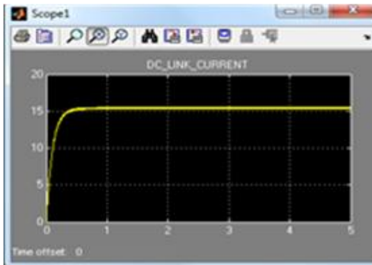
Fig. 5: (a) source voltage waveform (b) source current waveform (c) dc link current (d) load current waveform
