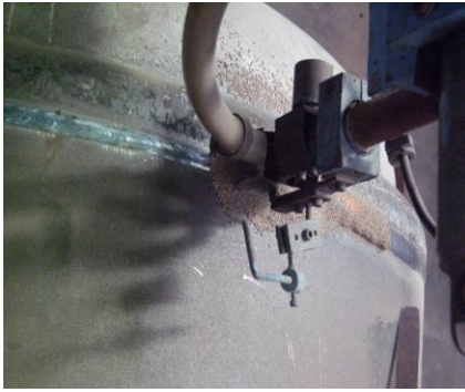
Figure. 1 Weld junctions of closure ring and jacket
