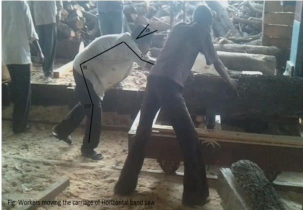
Fig 6. Workers manually moving the carriage
