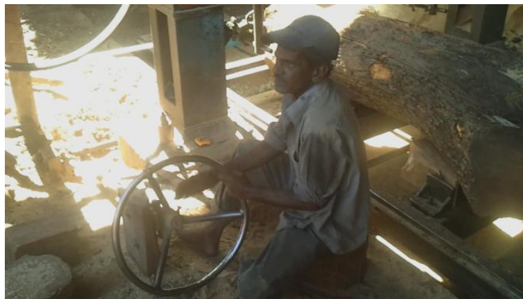
Fig 5. Worker moving the carriage of band saw using lever
