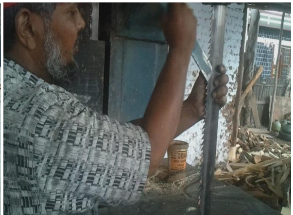
Fig. 11 Worker giving zigzag pattern to the saw blades
