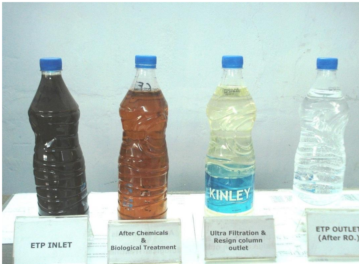
Figure 7: Difference in the colour of the coal gas based producer effluent after reverse osmosis in the ETP
