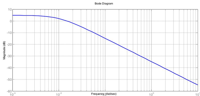
Fig.7 Magnitude plot of the spherical tank system
