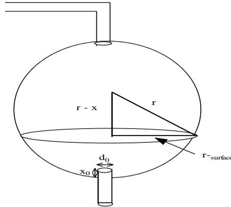
Fig. 1 Spherical Tank Level System
