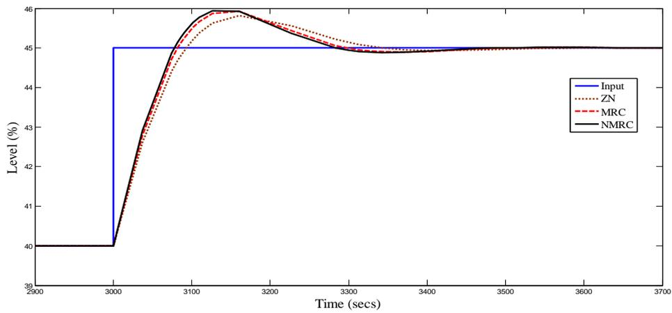
Fig.13 Tracking response of different controllers at operating range of 40 % with 5 % step change
