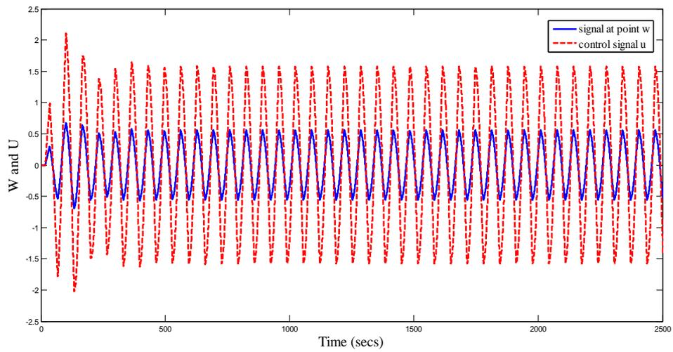
Fig.12 U and W signals based on MRC structure used for identification of controller parameters
