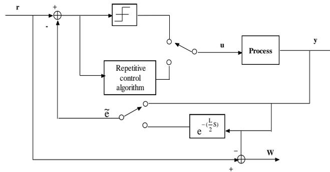
Fig. 3. Repetitive control algorithm with relay feedback.
