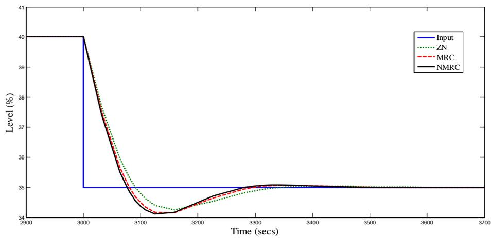
Fig.14 Tracking response of different controllers at operating range of 40 % with -5 % step change
