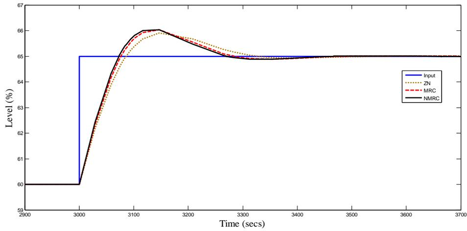
Fig.15 Tracking response of different controllers at operating range of 60 % with 5 % step change
