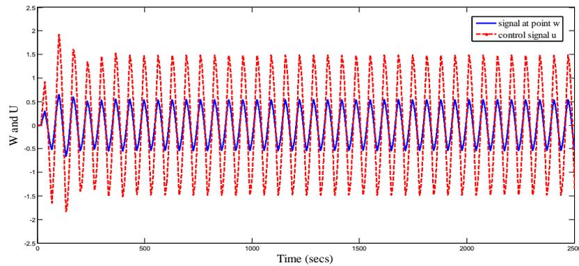
Fig.11 U and W signals based on MRC structure used for identification of controller parameters
