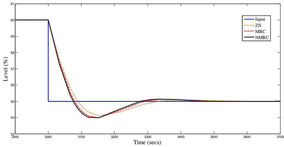
Fig.16 Tracking response of different controllers at operating range of 60 % with -5 % step change
