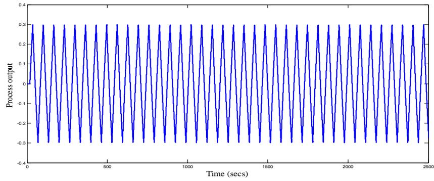
Fig.8 Output response of the process under relay feedback
