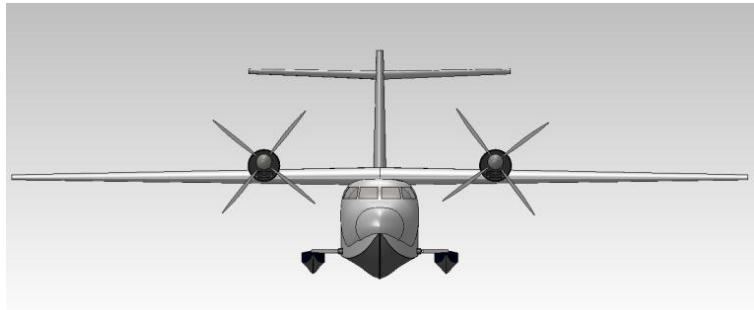
**Fig. 9:** CAD Model of Amphibian with Trimaran Concept
