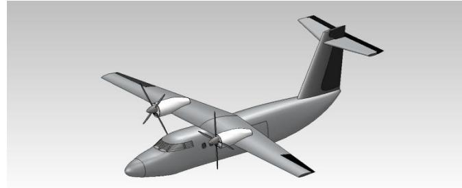
**Fig. 6:** 3-D CAD Model of Conventional Landplane Aircraft
