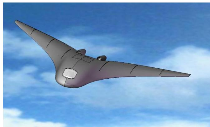
**Fig. 17:** Blended Wing Body Aircraft
