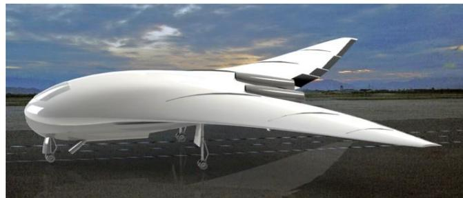
**Fig. 21:** Futuristic 3-D CAD Model of BWB Trimaran Amphibian
