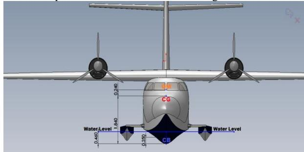
Fig. 11: CAD Model of Trimaran Seaplane at Transverse showing Metacentre, Centre of Gravity, and Buoyancy
