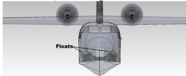
**Fig. 16:** Example CAD Model with undercarriage Floats
