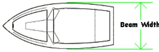
**Fig. 1:** Beam Width of a Conventional Boat [9]
