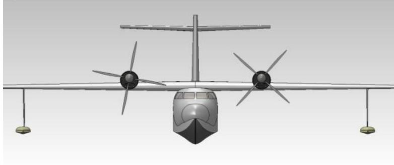
Fig. 7: CAD Model of Amphibian with Wing Tip Floats
