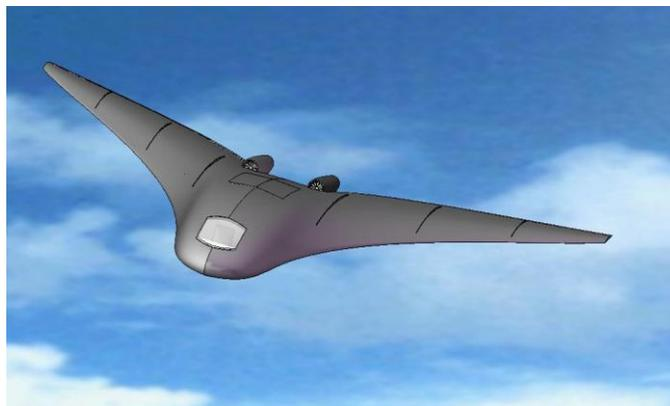
Fig. 17: Blended Wing Body Aircraft
