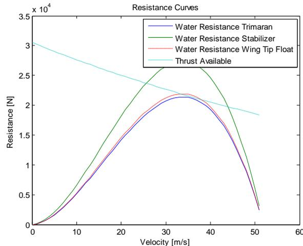
Fig. 12: Water Resistance Curves and Thrust Available
