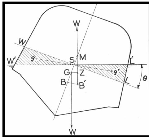
**Fig. 2:** Transverse Metacentric Height [2]
