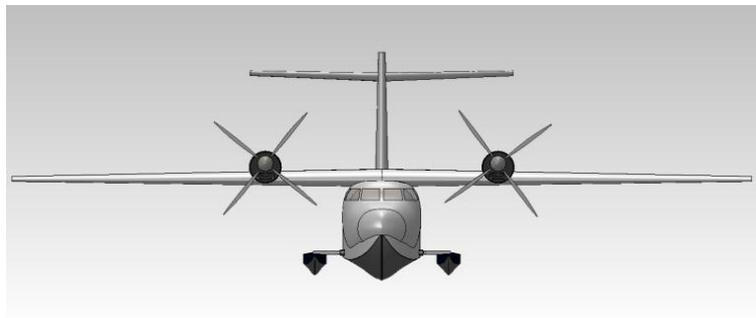
Fig. 9: CAD Model of Amphibian with Trimaran Concept
