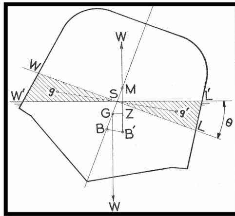
Fig. 2: Transverse Metacentric Height [2]
