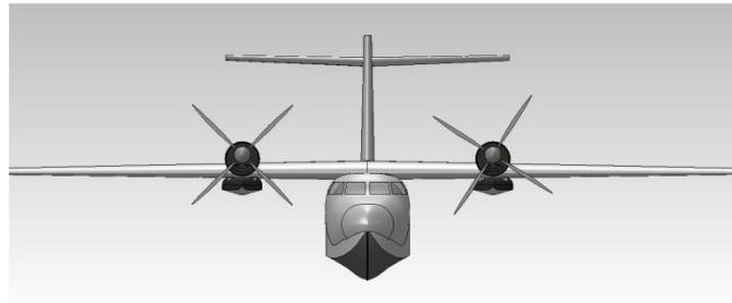
**Fig. 14:** Nacelle Wing Stabilizers Retracted
