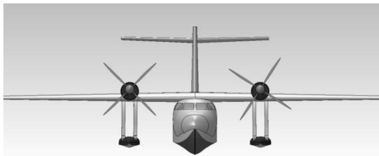
**Fig. 8:** CAD Model of Amphibian with Nacelle Support Stabilizers
