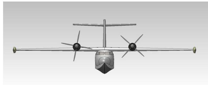
**Fig. 13:** Wing Tip Floats Retracted into the Wing Tips
