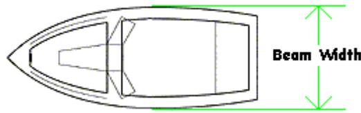
Fig. 1: Beam Width of a Conventional Boat [9]
