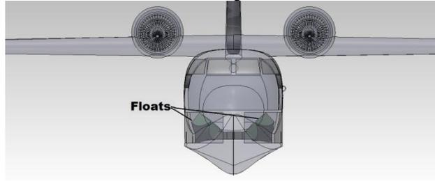
Fig. 16: Example CAD Model with undercarriage Floats
