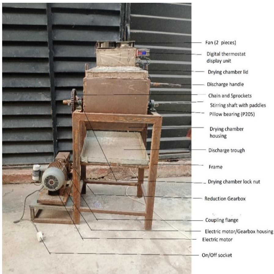
Plate 3. Pictorial view of the electric paddle grain dryer
