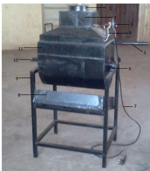
Plate 1. Pictorial view of the existing electric paddle grain Dryer
