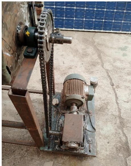
Plate 2. Arrangement of electric motor, gear box and stirrer shaft, sprocket, and chain
