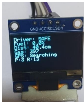
Fig.4. OLED display showing the real-time system monitoring status under normal operating conditions.
