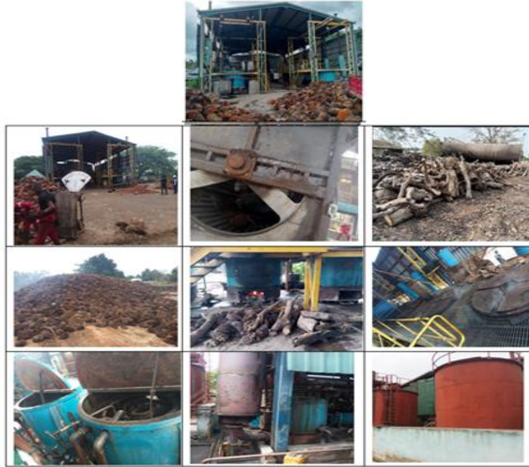
Figure 1: Crude palm oil mill plant with processing stages fruit reception, weighing of fruits, threshing of fruit bunch, furnace, cooking of fruit with wood/EFB, clarifier, dryer and Oil storage
