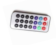
Figure 7: The NEC IR remote for controlling the mower movement
