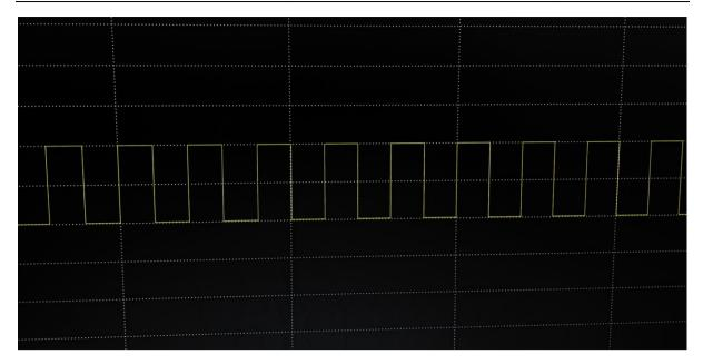
Figure 6: Inverter Output with RL Load
