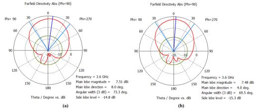
Figure 19: Antenna directivity at 3.6 GHz in H-plane (φ = 90°) (a) 2x1 MIMO antenna (b) 2x2 MIMO antenna
