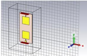
Figure 3: Designed 2 × 1 MIMO antenna using CST studio
