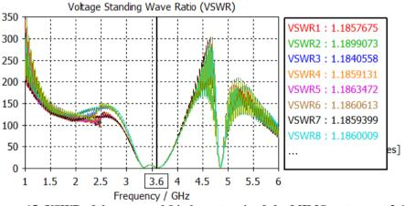
Figure 15: VSWR of the proposed 84-element series-fed mMIMO antenna at 3.6 GHz
