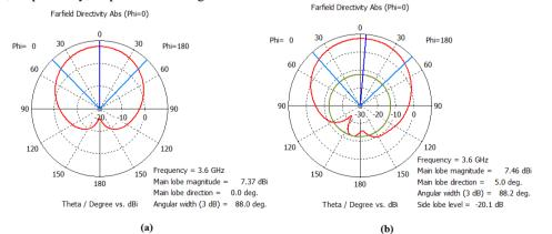
Figure 22: Antenna directivity at 3.6 GHz in E-plane ( $\varphi = 0^{\circ}$ ) (a) 2x1 MIMO antenna (b) 2x2 MIMO antenna
