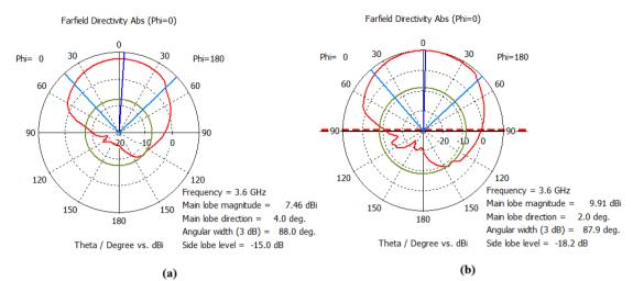
Figure 23: Antenna directivity at 3.6 GHz in E-plane ( $\varphi = 0^{\circ}$ ) (a) 40-element MIMO antenna (b) 84element mMIMO antenna
