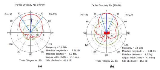
Figure 20: Antenna directivity at 3.6 GHz in H-plane ( $\varphi = 90^{\circ}$ ) (a) 40-element MIMO antenna (b) 84element mMIMO antenna
