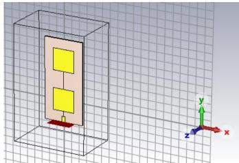
Figure 6: Designed 2 × 1 series-fed antenna using CST studio
