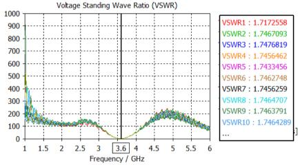
Figure 14: VSWR of the 40-element mMIMO antenna 3.6 GHz
