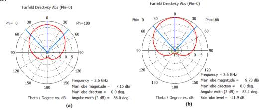
Figure 21: Antenna directivity at 3.6 GHz in E-plane (φ = 0°) (a) QWT-fed single patch (b) 2x1 series-fed patch
