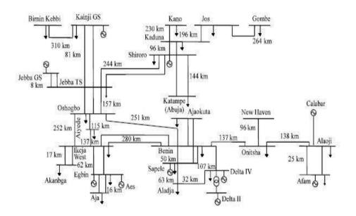
Figure 2: Single line diagram of the Nigeria 28 bus, 330kV transmission grid (Fasina et al, 2020)
