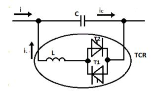
Fig 1. TCSC Controller (Meghwal and Mubeen, 2015).
