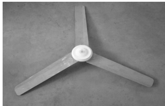
Fig.6.2 Composite Ceiling Fan Blade
