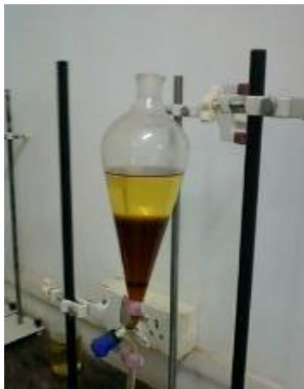
Fig. 9 The formation of glycerol (the red layer at the bottom) and FAME or biodiesel (the yellow layer at the top) by transesterification
