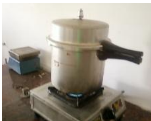
Fig. 8 Pressure cooking of de-feathered chicken skin immersed in water (this mixture is poured into an Aluminium vessel inside the pressure cooker) to form an organic layer, solid layer, and an aqueous layer.
