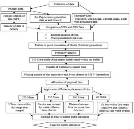
Fig. 6. Conceptual flow of the placement of community bins.
