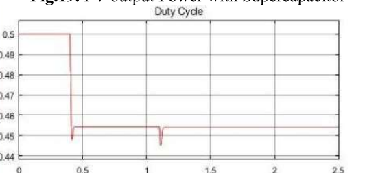
Fig.20. Duty cycle of boost converter with Supercapacitor
