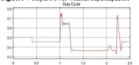
Fig.11. Duty cycle of boost converter without Supercapacitor
