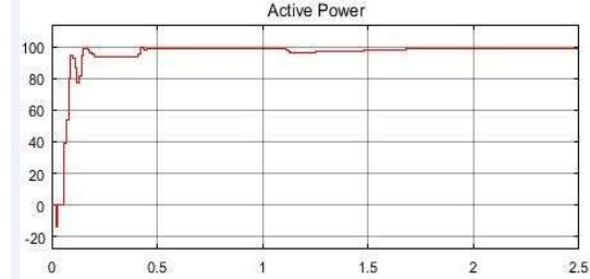
Fig.23. Activer Power transferred to the grid with Supercapacitor
