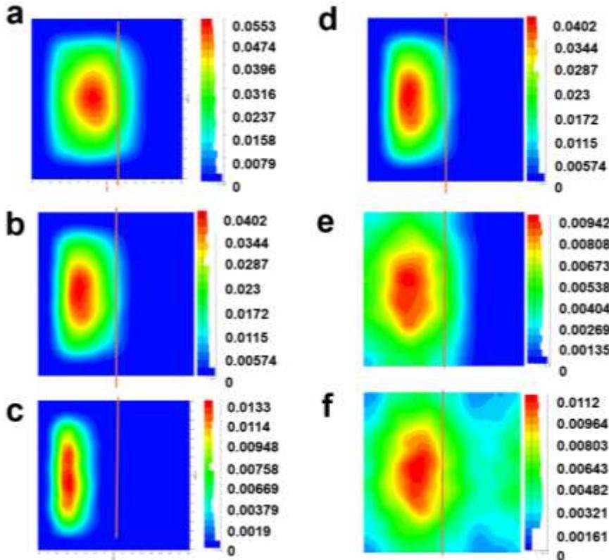
**Fig. 4.** Optical simulation results with prism angles of (a)  $30^\circ$ , (b)  $45^\circ$  and (c)  $60^\circ$  in zero tilting angle. And the results with tilting angles of (d)  $0^\circ$ , (e)  $15^\circ$  and (f)  $30^\circ$  when the prism angle is fixed to  $45^\circ$ .
