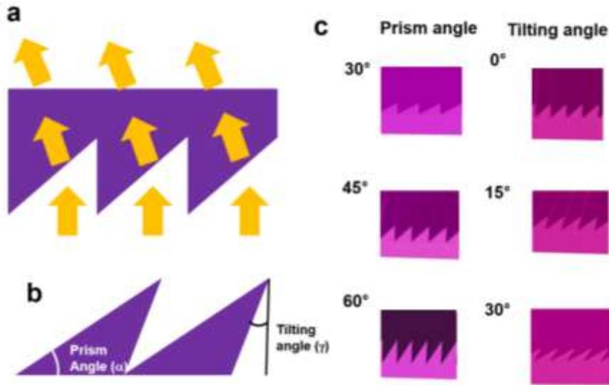
**Fig. 1.** a) A schematic of the directional transmission through asymmetric ratchets. b) Definition of prism angle and tilting angle. c) Designs for the experiment.
