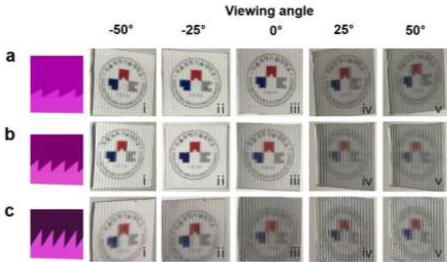
**Fig. 2.** Images of university logos through the transparent ratchet arrays with different viewing angle of  $-50^\circ$ ,  $-25^\circ$ ,  $0^\circ$ ,  $25^\circ$ , and  $50^\circ$  when the prism angle is (a)  $30^\circ$ , (b)  $45^\circ$  and (c)  $60^\circ$ .
