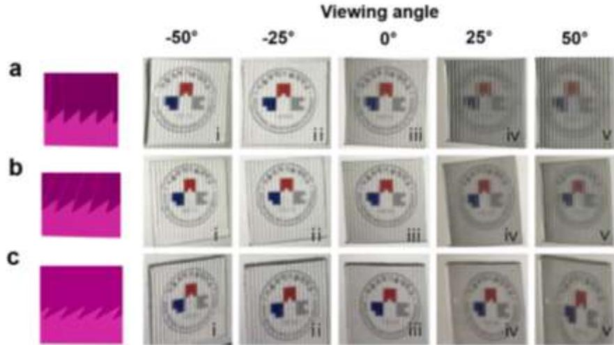
**Fig. 3.** Images of university logos through the transparent ratchet arrays with different viewing angle of  $-50^\circ$ ,  $-25^\circ$ ,  $0^\circ$ ,  $25^\circ$ , and  $50^\circ$  when the tilting angle is (a)  $0^\circ$ , (b)  $15^\circ$  and (c)  $30^\circ$ .
