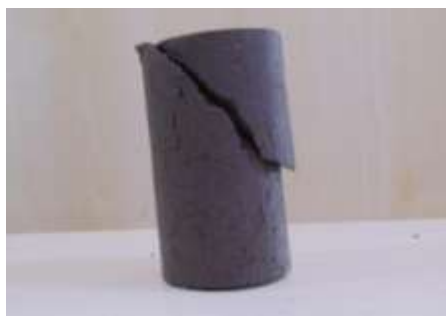
(a) Failure pattern of untreated soil sample
