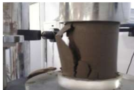
(b) Failure pattern of RBI treated soil sample X with 6% RBI and 28 days curing period
