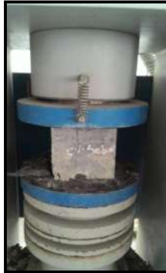
Fig 1: Compressive Strength Test
