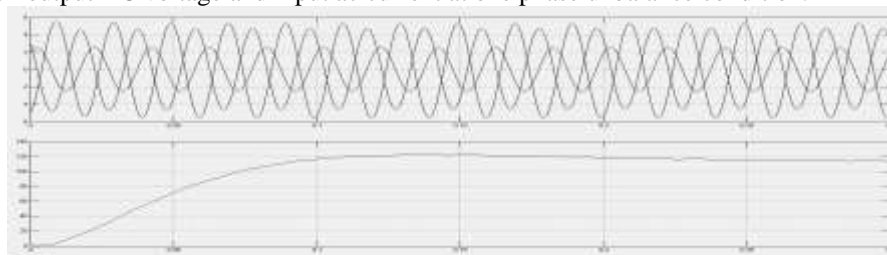
Fig4: case2 output DC voltage and input ac current at one phase unbalance condition.
