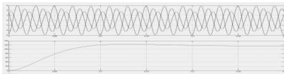
Fig6: case4 output DC voltage and input AC current at three phase unbalance condition.
