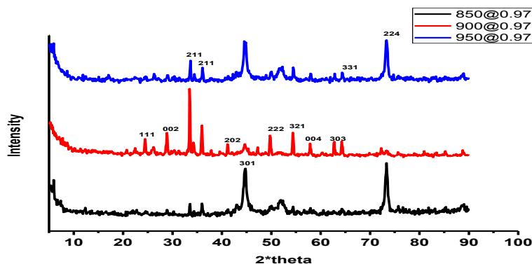
XRD graphs of PPy/Ti-doped barium ferrite at  $850^{\circ}\text{C}$ ,  $900^{\circ}\text{C}$  and  $950^{\circ}\text{C}$  temperatures
