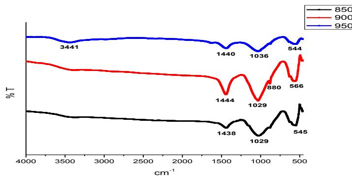
**Fig 3** FT-IR images of PPy/Ti-doped barium ferrite at 850°C, 900°C and 950°C temperatures
