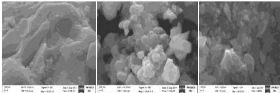
**Fig 2** SEM images of PPy/Ti-doped barium ferrite at 850°C, 900°C and 950°C temperatures
