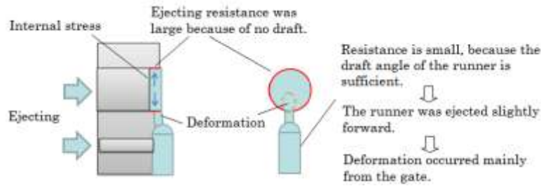
Fig.16: Mechanism that the in-mold residual pressure causes the deformation of sample
