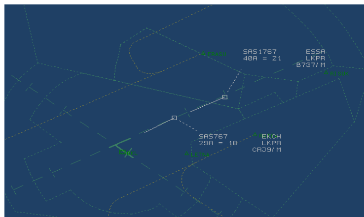
Figure 4 – Radar screen with similar call-signs (flights SAS767 and SAS1767) on final RWY 24 at LKPR
