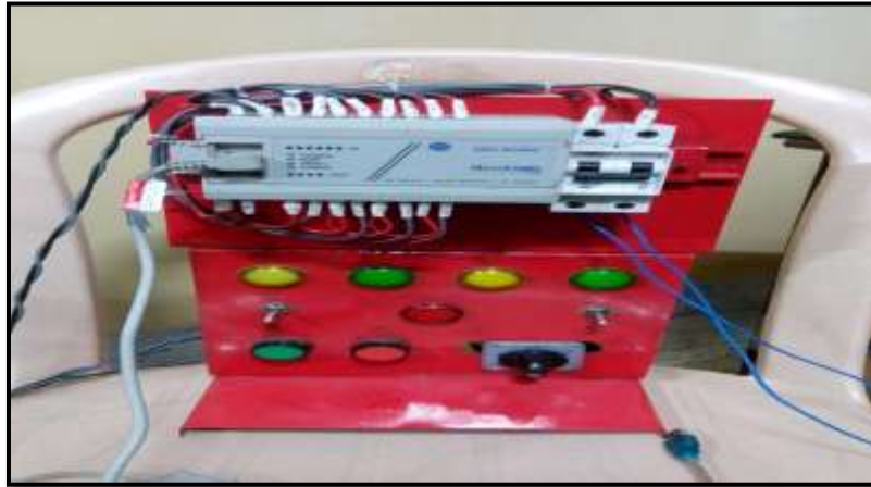
Fig1: The snapshot of the PLC micrologix 1000
