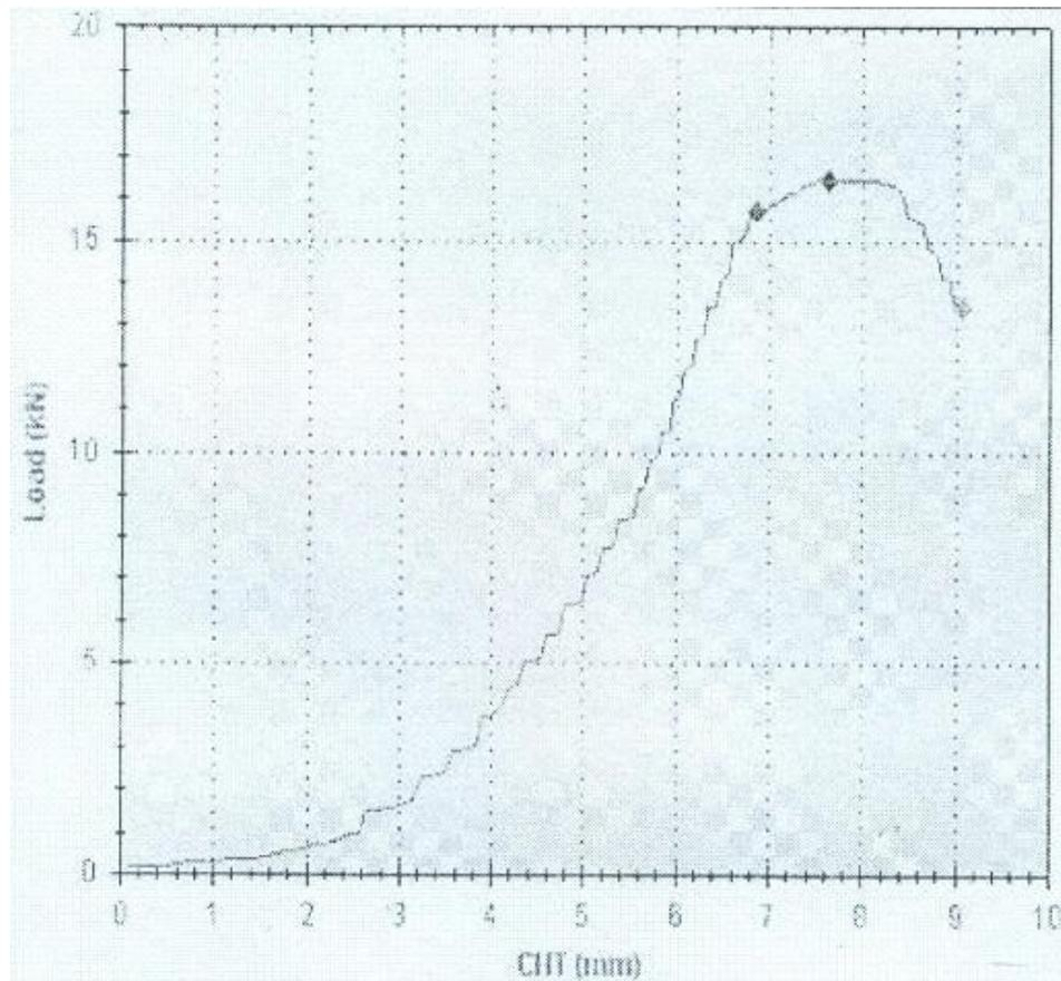
**Fig.2: Load vs. Elongation curve for SLM Ti-6Al-4V test coupon after heat treatment According to AMS 4928 standard**
