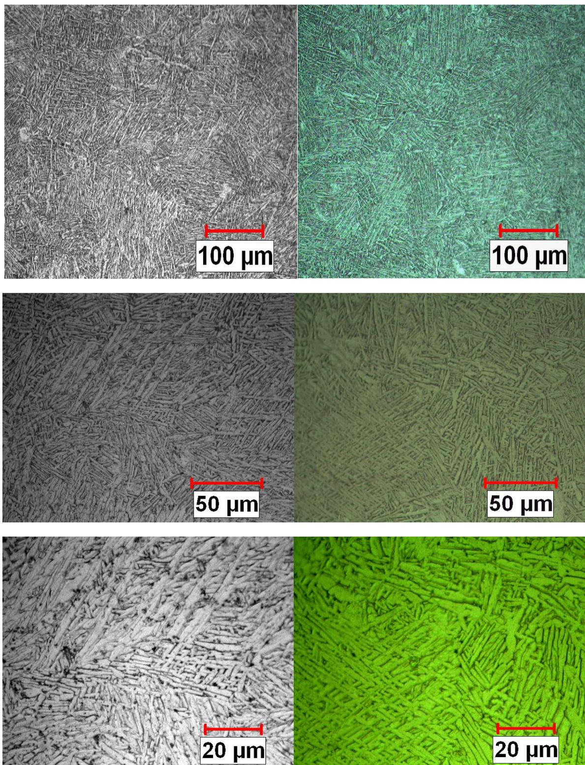
Fig.3: Microstructure images of Ti-6Al-4V at 200X, 500X and 1000X respectively after heat treatment with AMS 4928 guidelines. Left side B/W for specimen 1 and right side colored for specimen 2.
