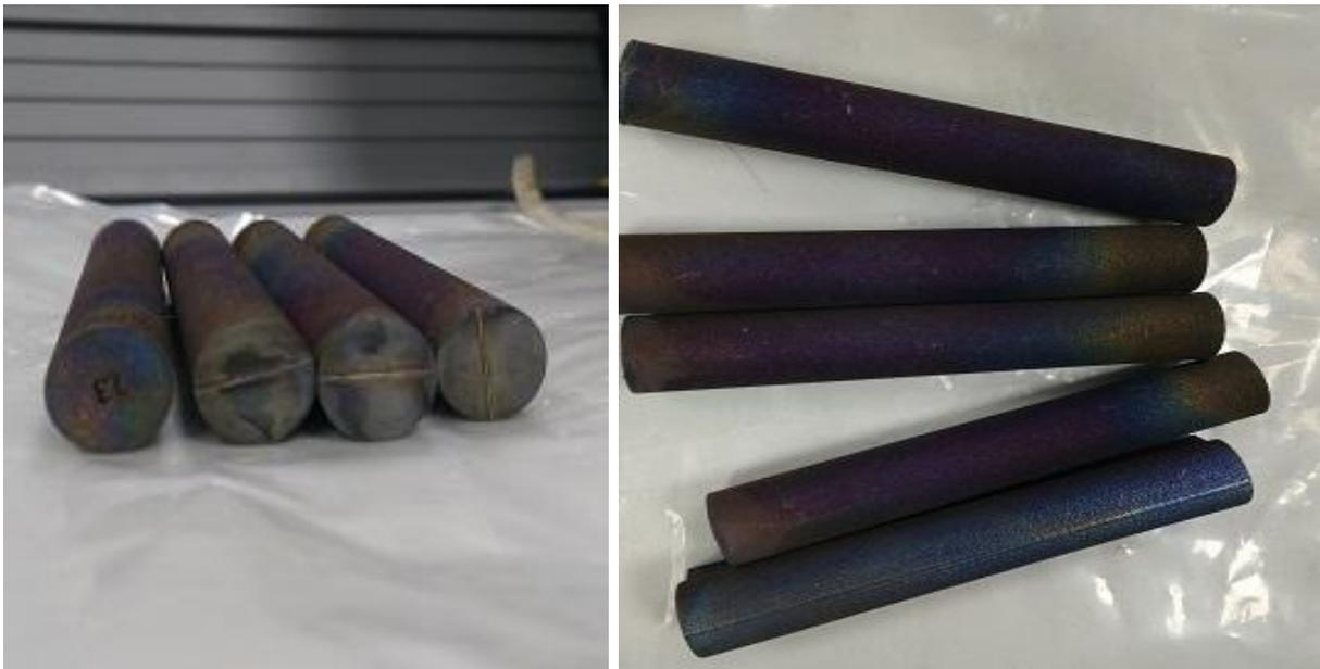
**Fig.1: Macroscopic Samples of Ti-6Al-4V test coupons prepared by SLM Method on EOSINT M 280 DMLS 3D Printer.**
