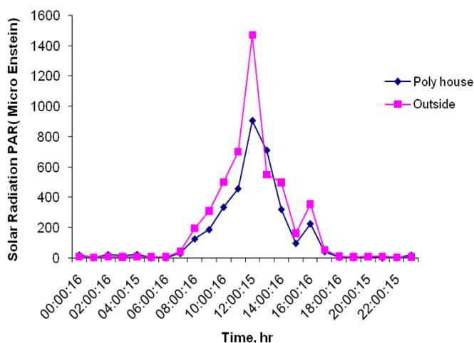
Fig.6: Variation of solar radiation in poly house and open field
