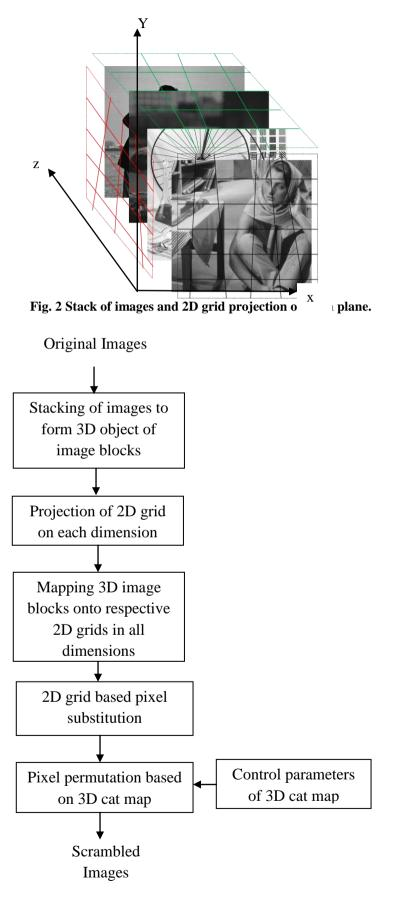
Fig. 3 Proposed Encryption Scheme
