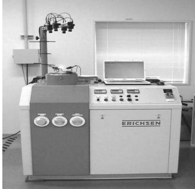
Fig. 1: Erichsen testing machine and measuring cameras
