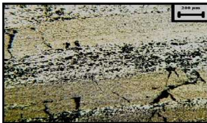
Fig. 4: Photomicrograph showing the the bands of specular hematite in hard laminated ore.
