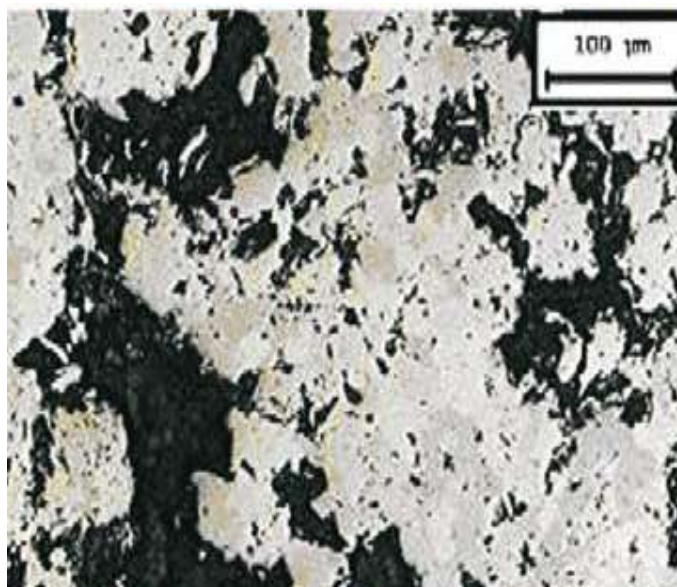
Fig. 5: Photomicrograph showing Martite in hard/massive iron ore.
