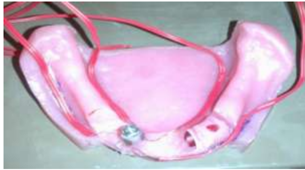
Fig. 2 : Model with installed implant and strain gauges.
