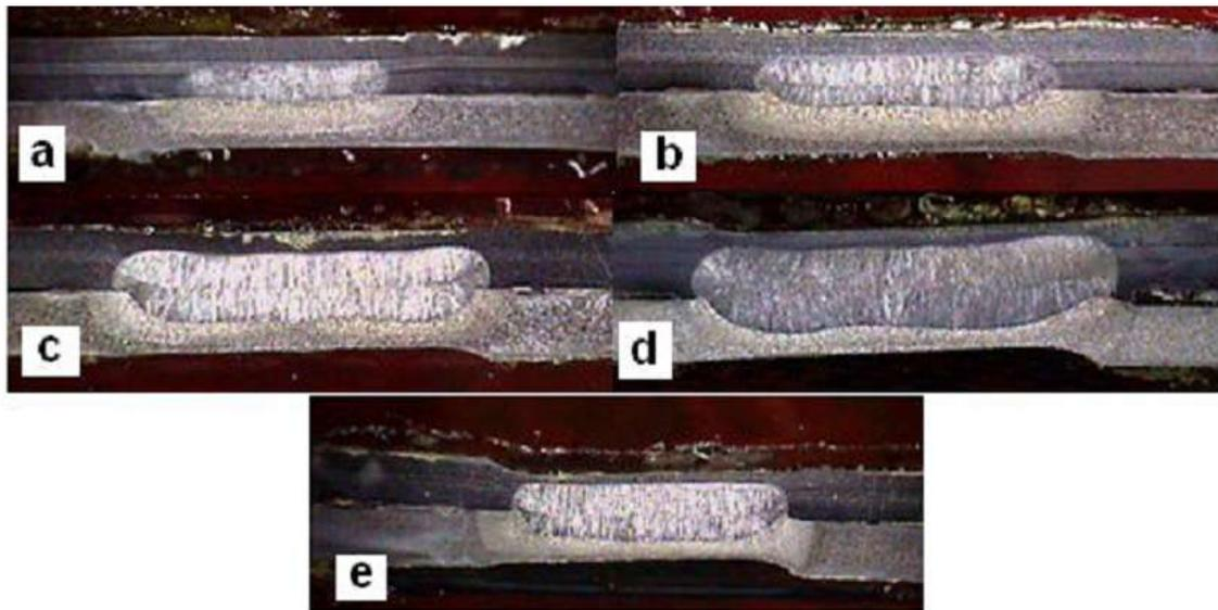
**Fig.3 Effect of welding current on the weld nugget growth: a) 8kA b) 9kA c) 10 kA d) 11kA**
