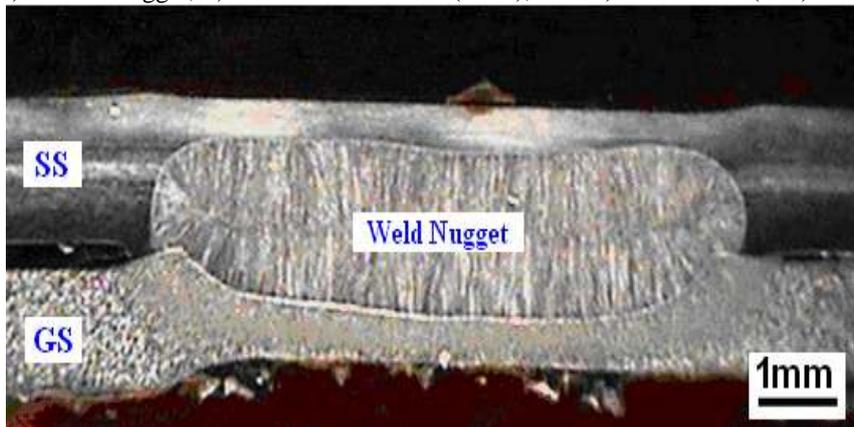
**Fig.2 Macrostructure of dissimilar RSW between galvanized steel and stainless steel**
