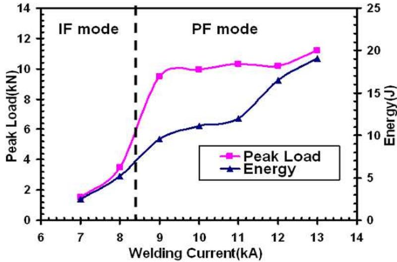
Fig.7 Effect of welding current on the peak load and failure energy
