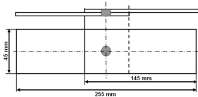
**Fig.1 Tensile-shear test sample dimension**
