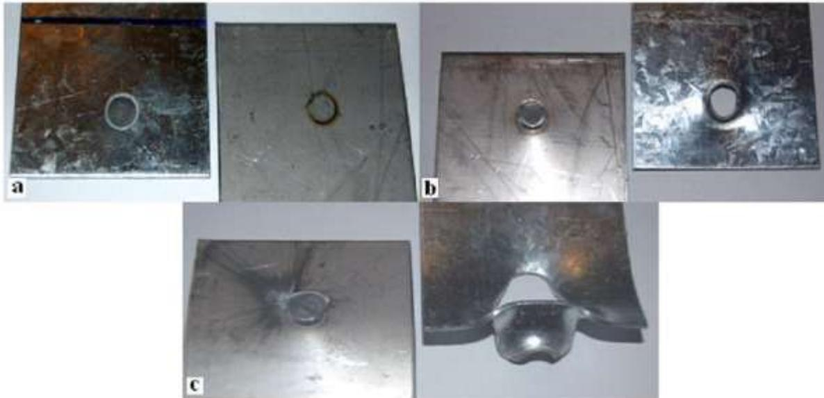
Fig.8 (a) Interfacial failure mode, (b) pullout failure mode and c) nugget pullout followed by Sheet tearing.
