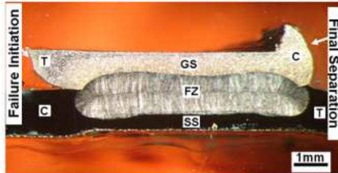
**Fig.9 Macrograph of fracture surface cross section, T: Subjected to tensile stress
