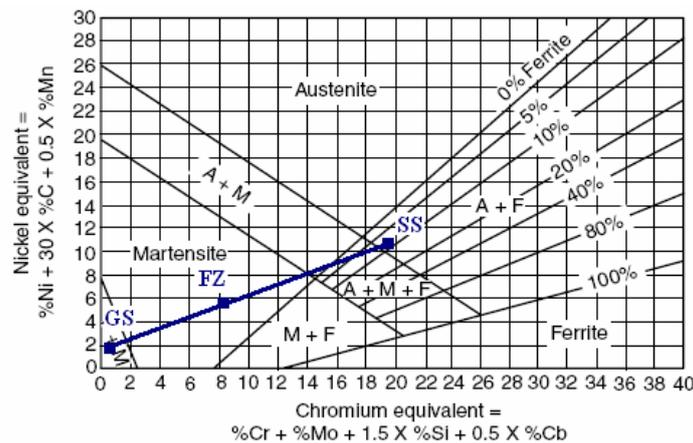
Fig.6 Schaeffler diagram, fusion zone microstructure prediction, when weld nugget consists of 60% galvanised steel
