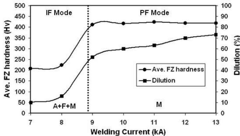
**Fig.4 Effect of welding current on the dillution, microstructure, average FZ hardness and Failure mode of the dissimilar joint**
