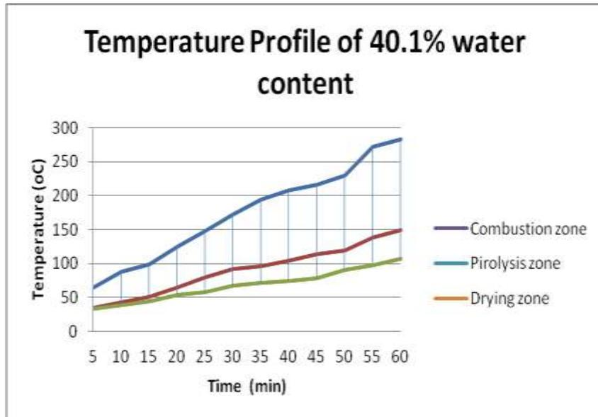
Fig. 3. Waste incineration temperature profile water content 40.1%
