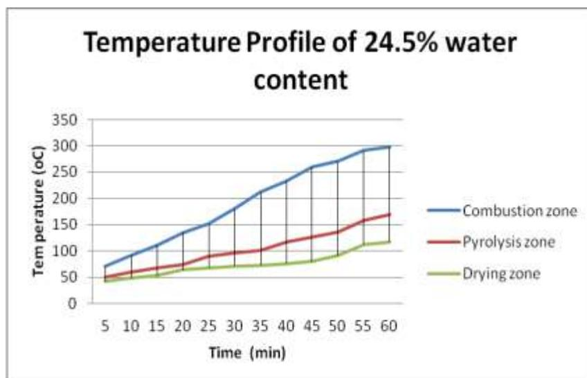
Fig. 5 Temperature Profile burning waste water content of 24.5%
