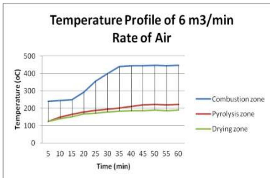
Fig. 9 Profile of temperature combustion water content of 15.1% with 6 air m<sup>3</sup>/minute
