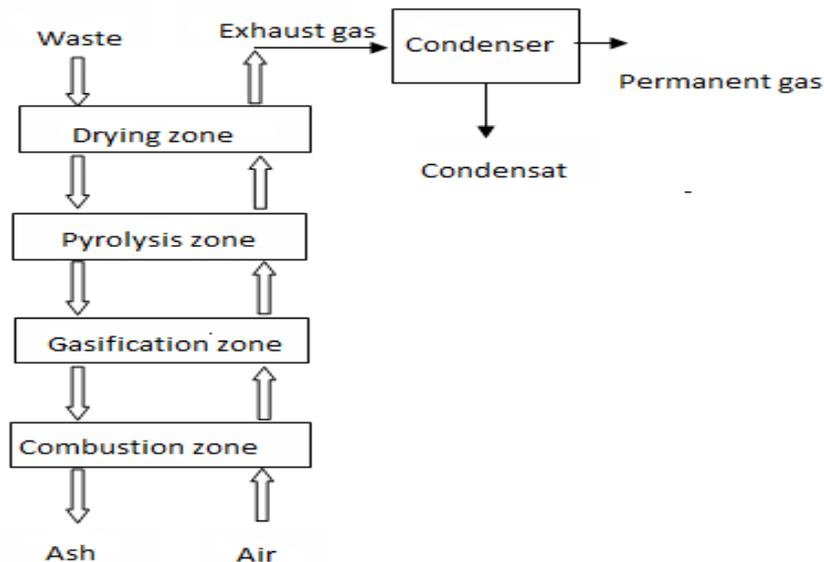
**Fig. 1. Various zones in the updraft fixed bed incinerator**
