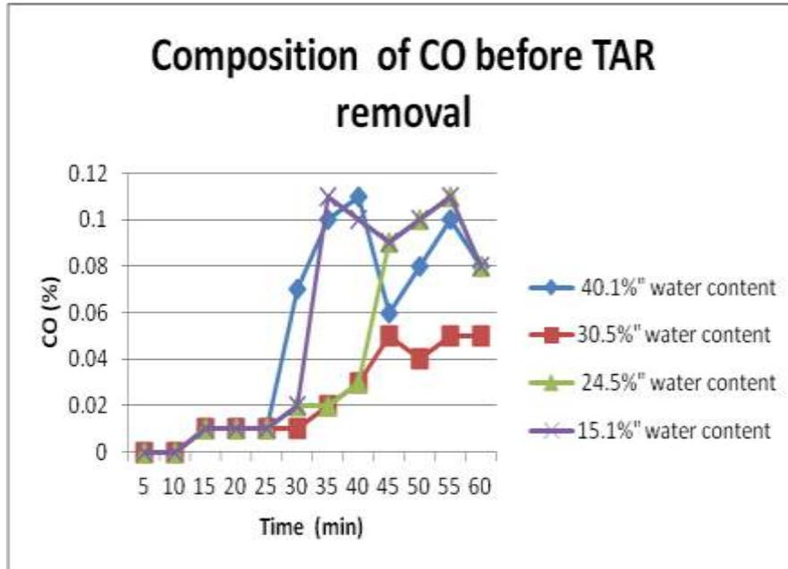
Fig .11 Composition CO in the flue gas before the separation of tar
