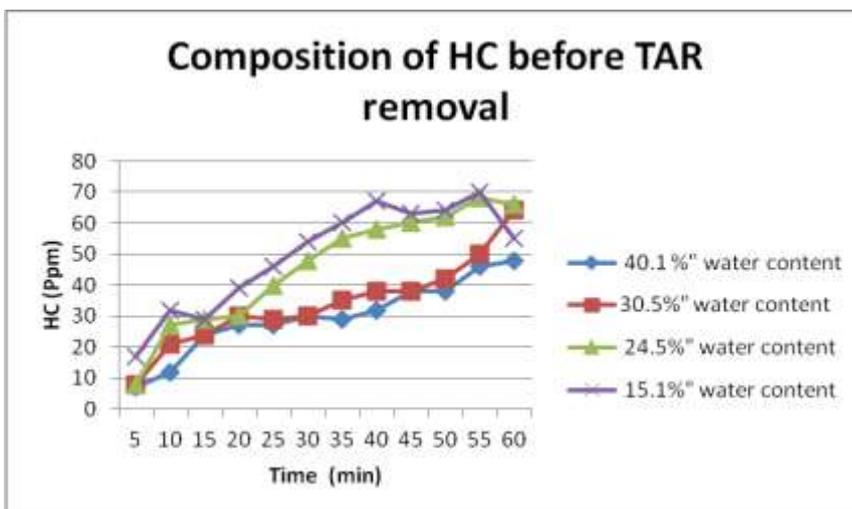
Fig. 15 Composition of HC in the exhaust gases before the separation of tar
