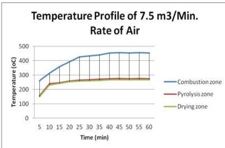
Fig. 10 Combustion temperature profile water content of 15.1% with 7.5 air m<sup>3</sup>/minute
