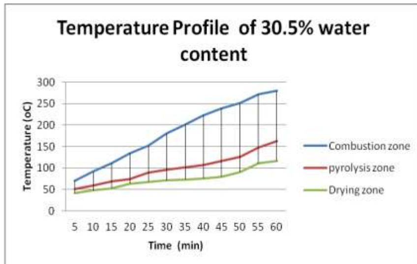
Fig. 4. Waste incineration temperature profile water content 30.5%
