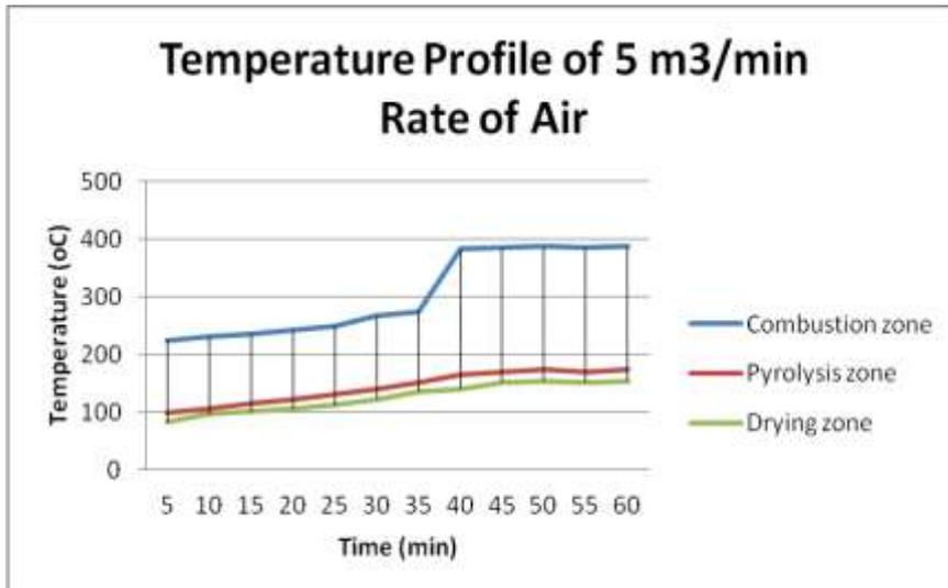
Fig. 8 Profile of temperature combustion with a water content of 15.1% air 5 m<sup>3</sup>/minute
