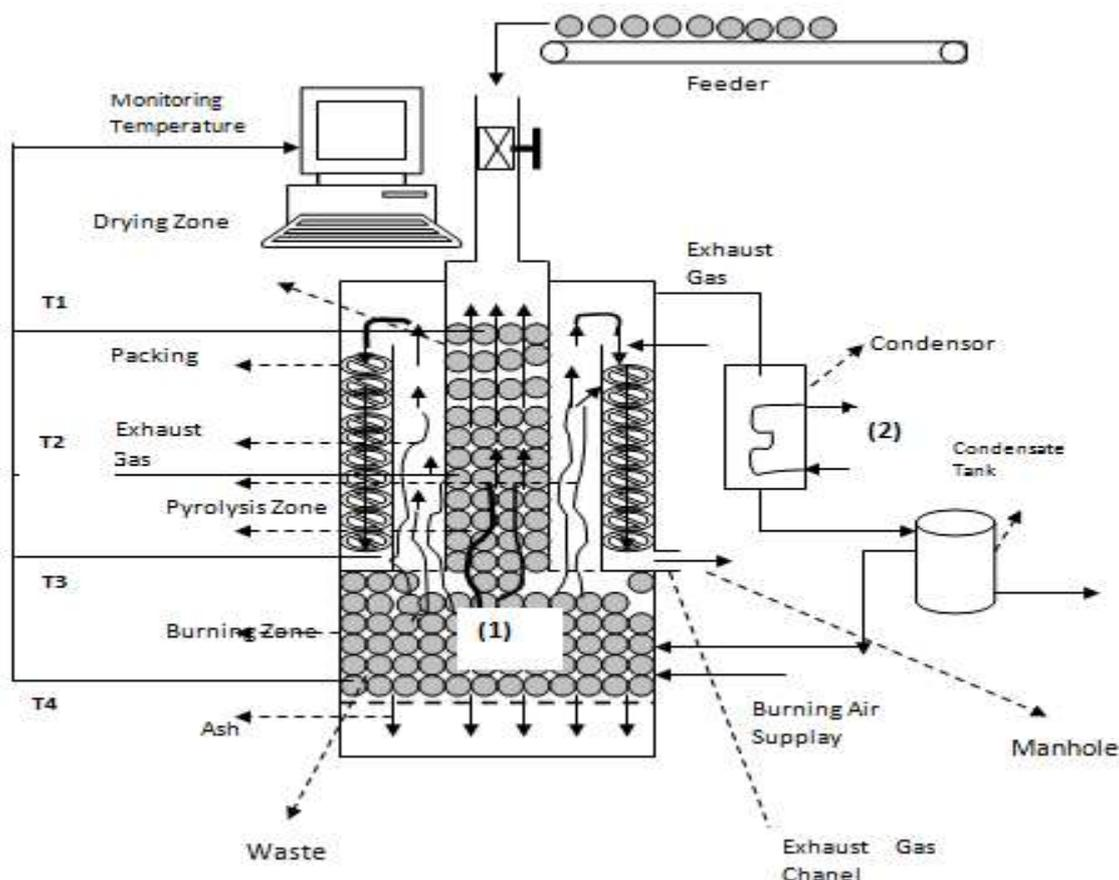
Fig. 2. Schemes of work equipment incinerator
