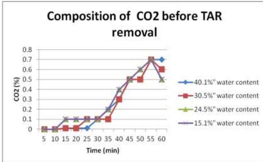
Fig.13 Composition of CO<sub>2</sub> in the flue gas before the separation of tar
