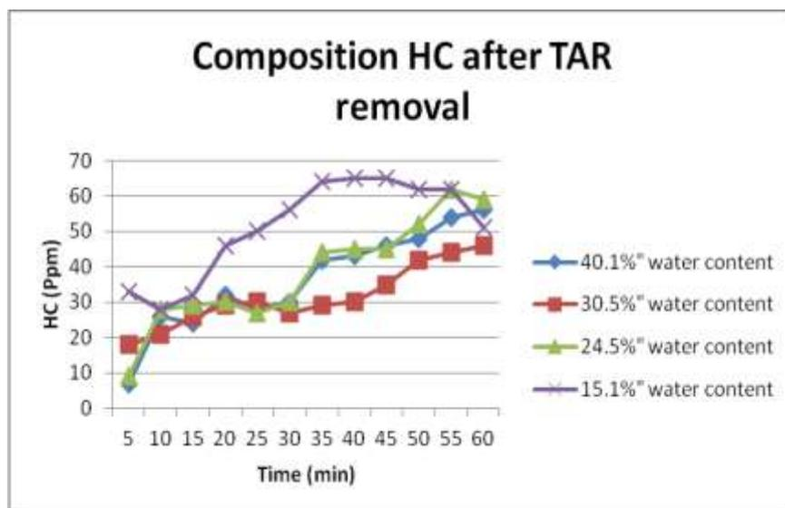
Fig. 16 Composition of HC in the exhaust gases after separation of tar
