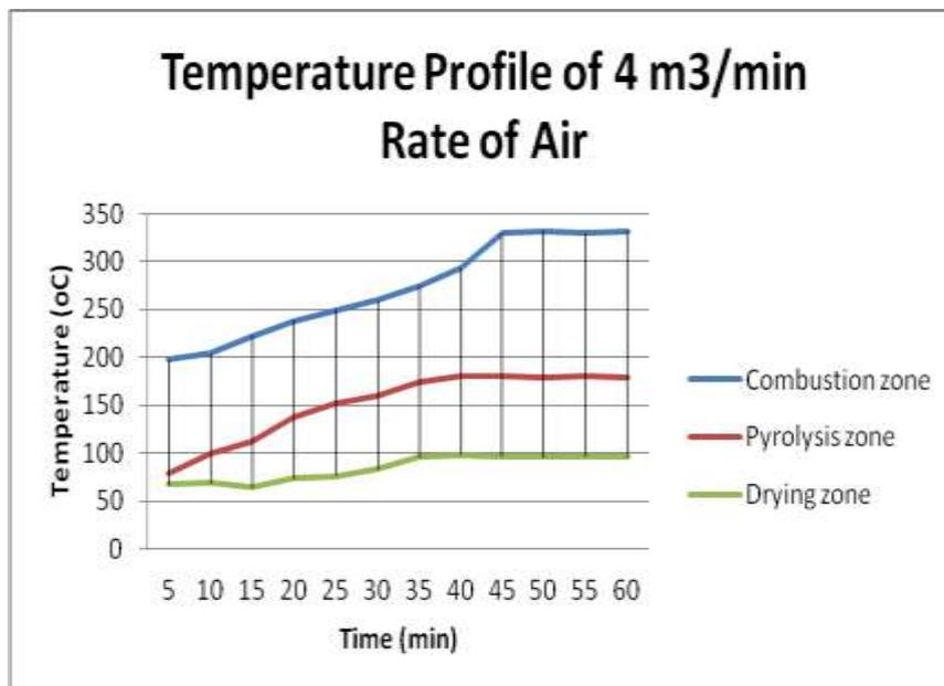
Fig. 7 .Profile of temperature combustion water content of 15.1% by air 4 m<sup>3</sup>/minute
