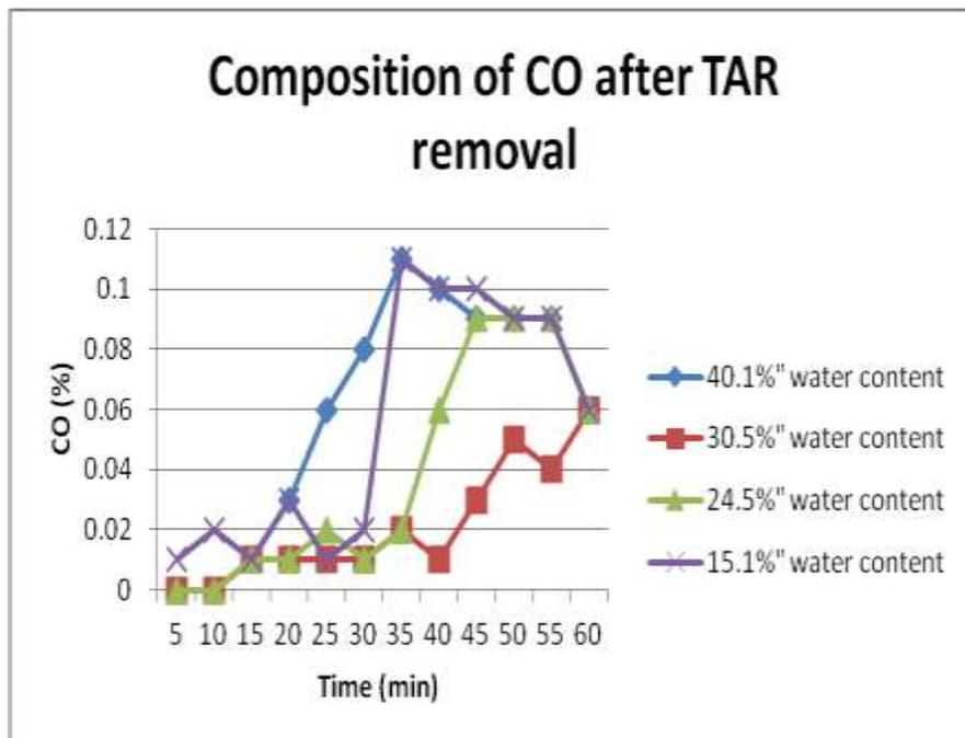
Fig.12 The composition of CO in the flue gas after the separation of tar.
