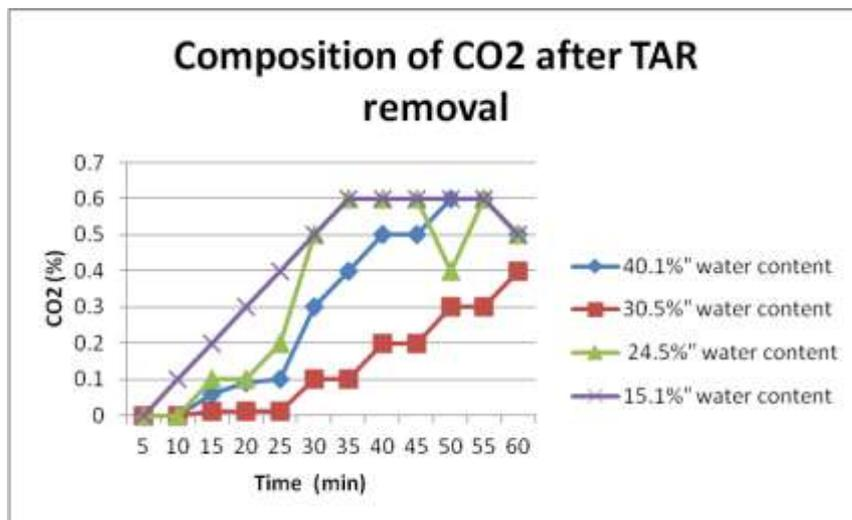
Fig. 14 Composition of CO<sub>2</sub> in the flue gas after the separation of tar
