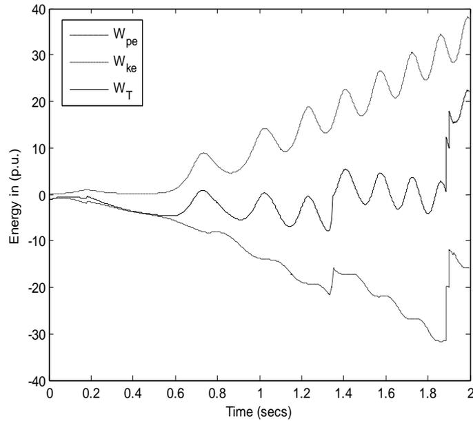
**Figure 4.2. Variation of Energy with time without HVDC**
