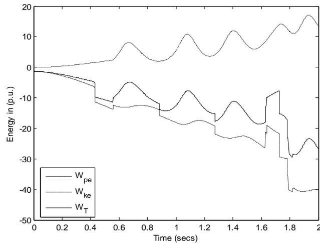
**Figure. 4.18. Variation of Energy with time without HVDC**
