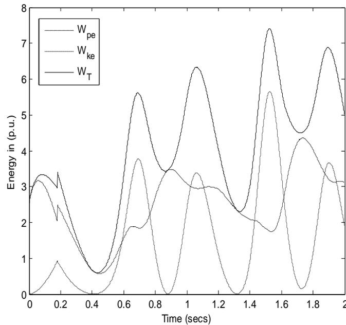
**Figure 4.3. Variation of Energy with time with HVDC**
