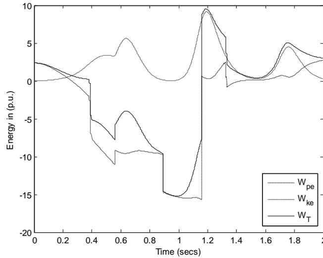
**Figure 4.19. Variation of Energy with time with HVDC**
