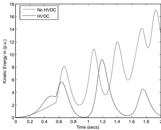
**Figure 4.21. Variation of kinetic energy with time**
