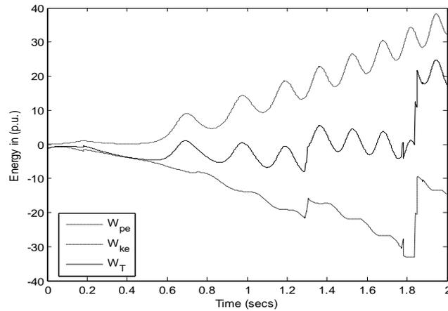
**Figure 4.10. Variation of Energy with time without HVDC**
