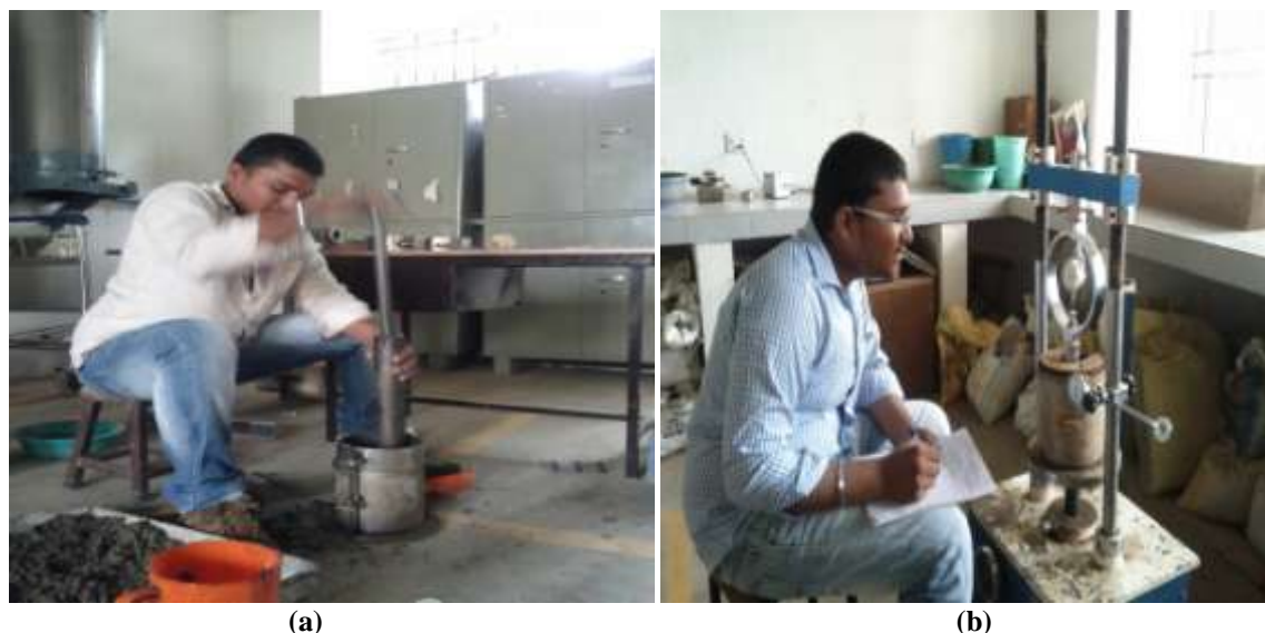
Fig II: (a)Preparation of sample by author for conducting CBR test (b)Author is performing CBR test
