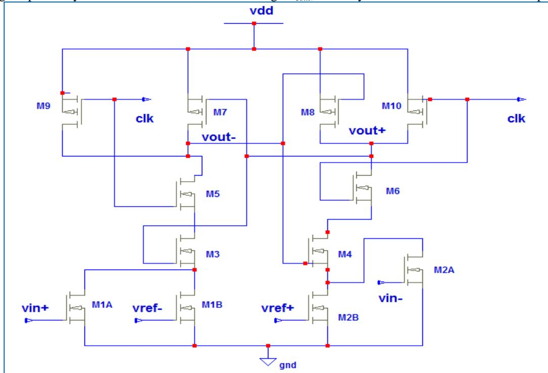
Fig 5: Lewis-Gray Comparator.(Comparator1)
