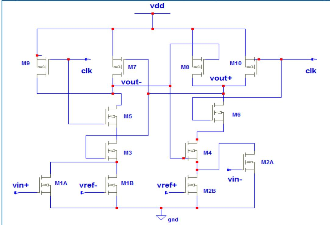
Fig 5: Lewis-Gray Comparator.(Comparator1)
