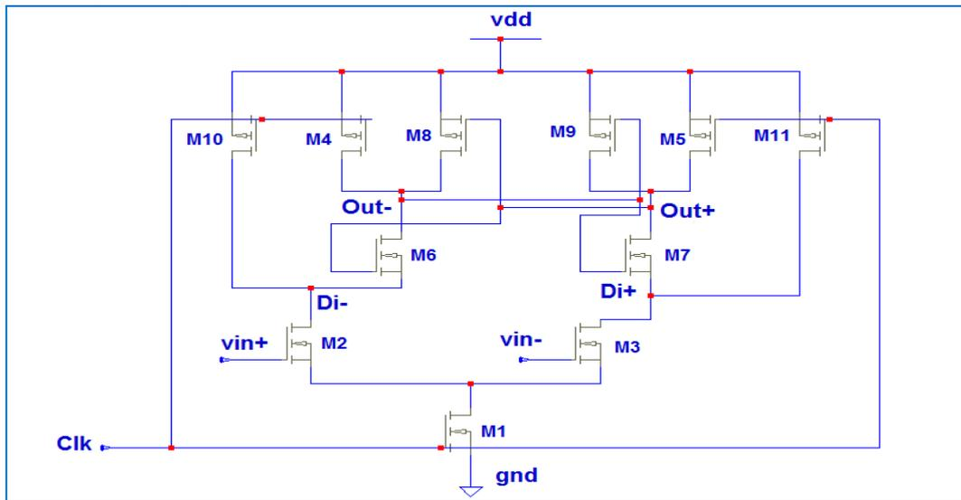
Fig 6: Latch-type Voltage SA .(Comparator2)
