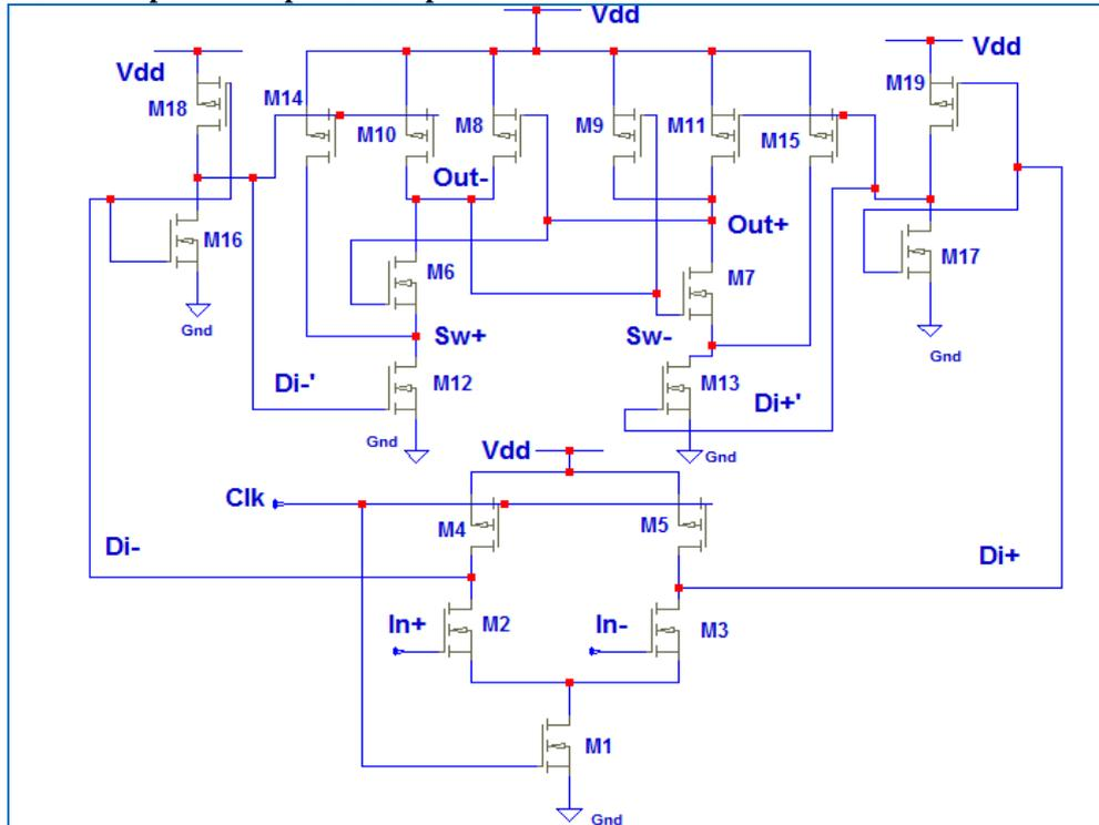
Fig 8 : Schematic of Proposed comparator.(Comparator4)
