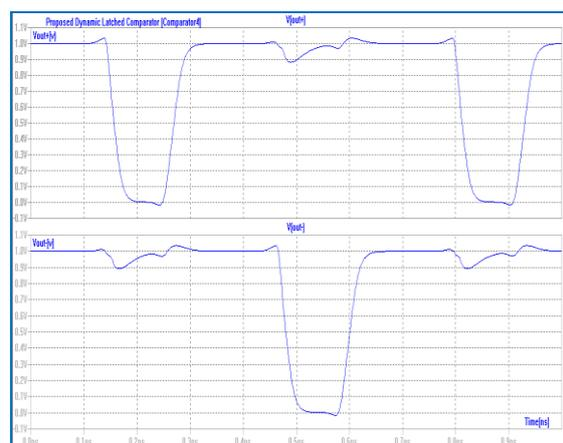
Fig 12: Proposed Dynamic Latched Comparator (Comparator4)
