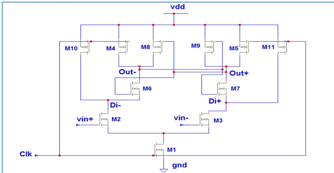
Fig 6: Latch-type Voltage SA .(Comparator2)
