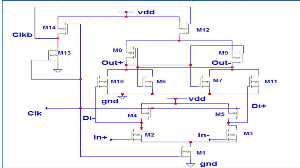
Fig 7: Double-Tail Dynamic Latched Comparators.(Comparator3)
