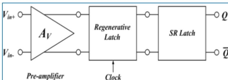
Fig 1: Typical block diagram of a high-speed voltage comparator.
