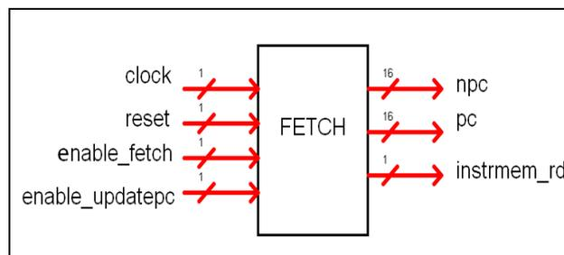
Figure 4: Entity diagram of the Fetch block.
