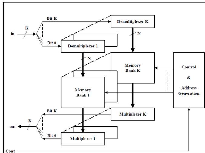
• **Figure1: Conventional DRFM architecture using standard components.**
