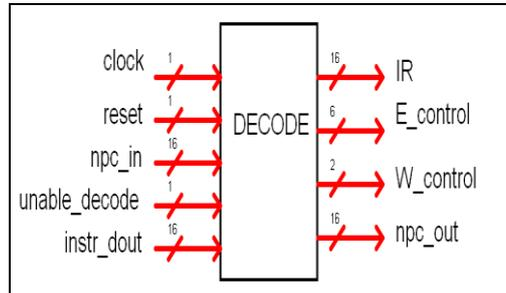
**Figure 5: Entity diagram of the Decode block.**
