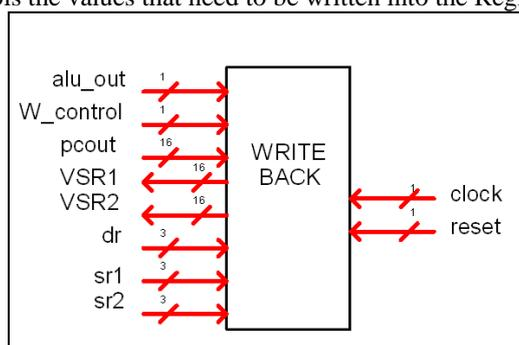
Figure 7: Entity diagram of the WriteBack block.
