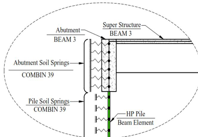
**Fig.10: Finite element modeling with ANSYS**
