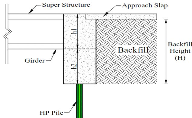
**Fig.2: Soil Backfill in Integral Abutment Bridge**
