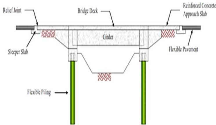
**Fig.1 Typically of Integral Abutment Bridges with HP pile**
