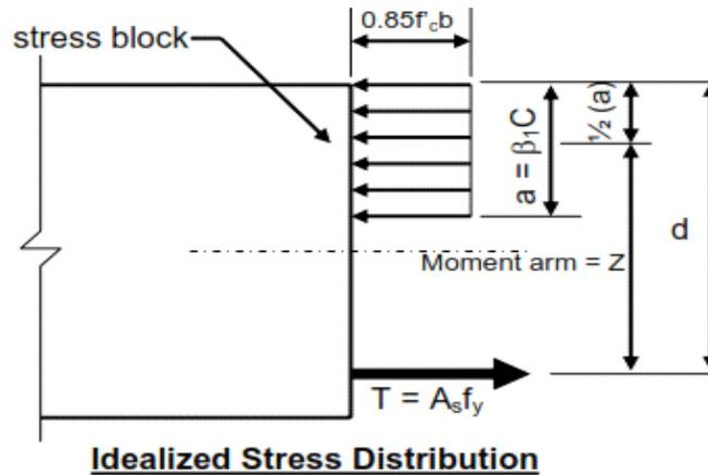
**Fig.4: Whitney's equivalent stress block**
