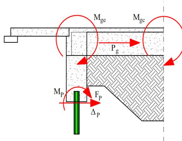
**Fig.12: Specific location in integral abutment bridge**
