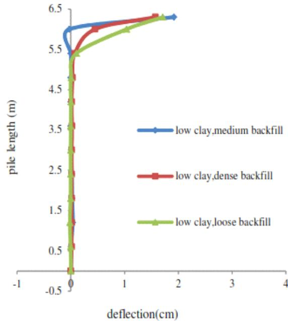
**Fig. 15: Lateral deflection of abutment case 7, 8, 9**
