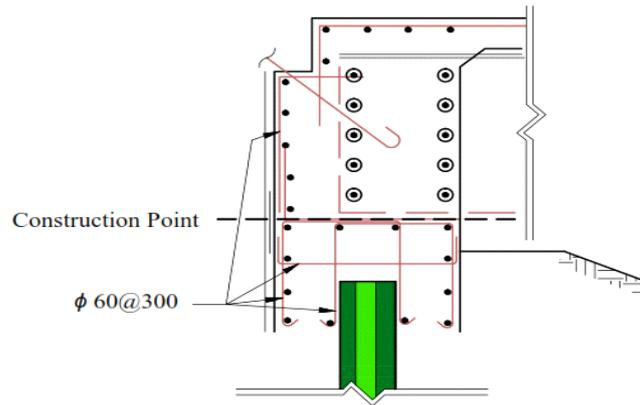
**Fig.5: Penn DOT Standard for Integral Abutment Details**
