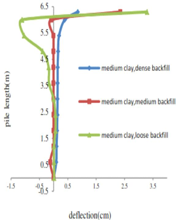
**Fig. 14: Lateral deflection of abutment case 4, 5, 6**
