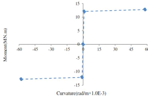
**Fig.6: Moment Curvature Relation for Penn DOT Detail**
