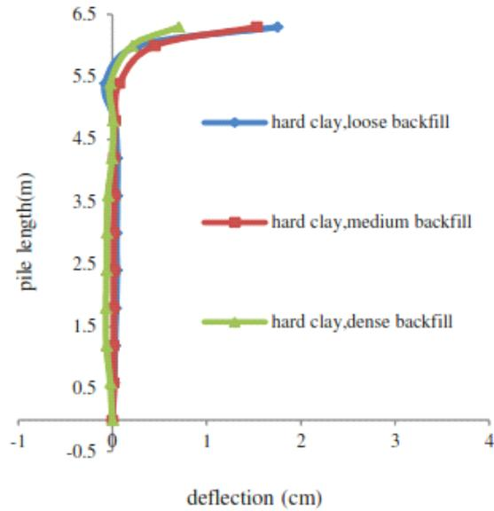
**Fig. 13: Lateral deflection of abutment case 1, 2, 3**
