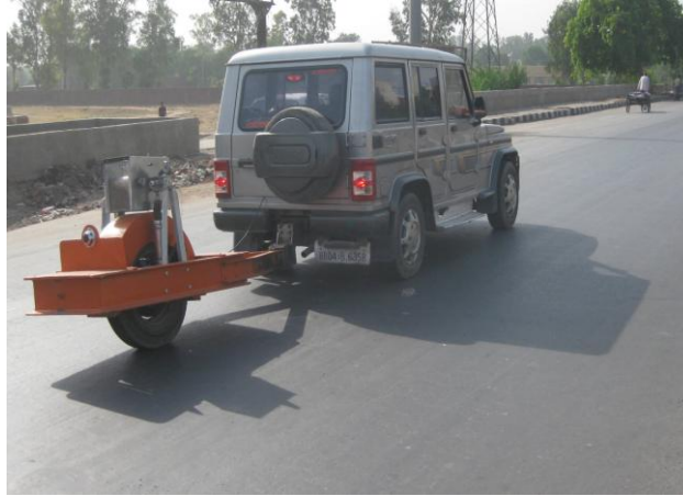
Figure 1. A View of Fifth Wheel Bump Integrator Measuring Surface Roughness
